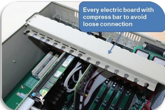
Every electric board with compress bar to avoid loose connection
