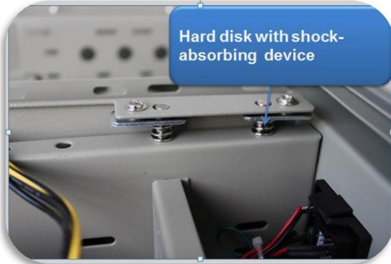
Hard disk with shock-absorbing device
